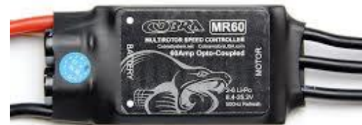
Figure 8 – Electronic Speed Controller [5]
