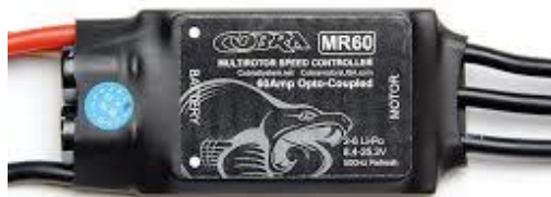
Figure 8 – Electronic Speed Controller [5]
